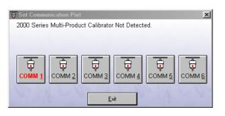
On starting the virtual front panel for the first time, a COM port selection screen will be displayed. Click on the COM port which is connected to your 2000 Series calibrator to continue.
